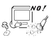
The ventilation holes prevent overheating. Do not block or cover these holes. Especially avoid covering the holes with soft materials such as cloth or paper.
